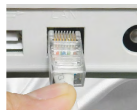
LAN cable connection
